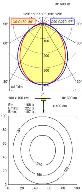
light source LED work equipment without connected load 22-26 V, DC power consumption env. 12,0 W luminous flux approx. 600 lm luminous efficiency approx. 50 lm/W
